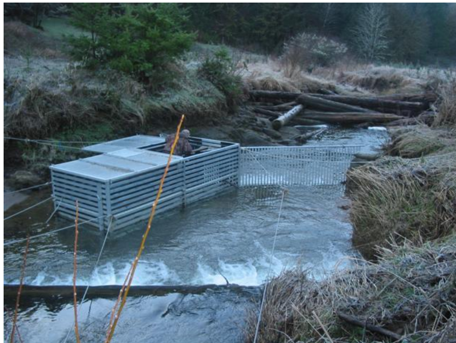
Figure 2. Fisher checking the Palouse adult trap for fish and clearing debris from the trap.
